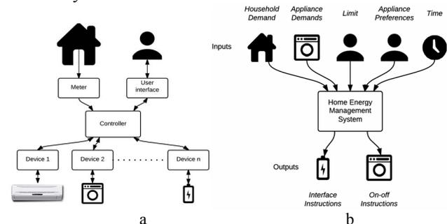
Figure 1: Structure of a Home Energy Management System (a) and inputs and outputs for demand tariff (b).
