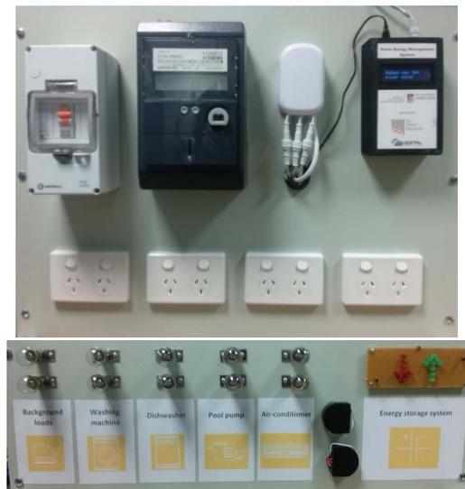
Figure 5. Demonstration frame circuit and load bank.
