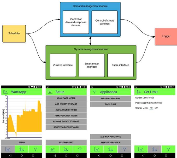
Figure 6 Overviews of the controller's software (top) and smartphone application screen shoots (bottom)
